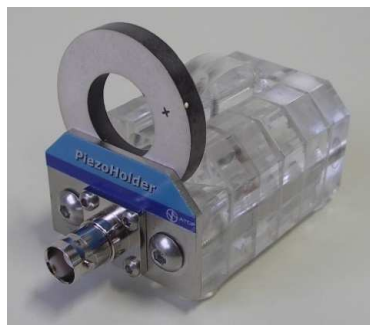
Figure 9 – PiezoHolder support for the connection between ceramics and the TRZ Analyzer.
