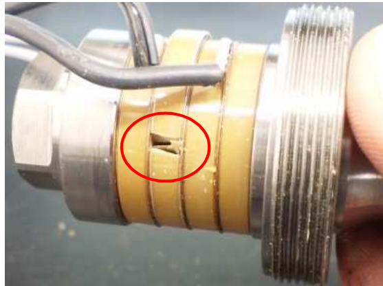
Figure 11 – Ultrasonic converter with a fractured piezoelectric ceramic piece. The other pieces were recovered and used after being tested for internal cracks.
